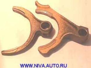
Worn out forks are replaced by new ones.
