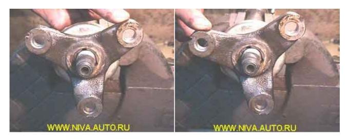
In my practice I found a case where the main shaft splines were damaged. On the left picture it is well visible how the splines were narrowed down. This was the result of a quite negligent attitude (operating the gearbox with a loose rear nut):
