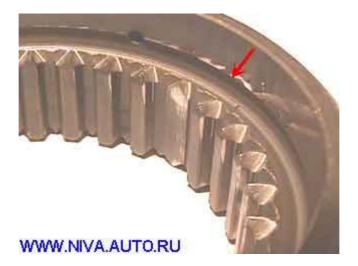
Examine the tooth end faces. They should be sharp without deterioration or chopped off:
