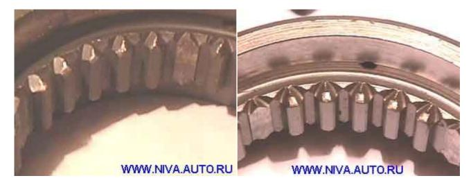
Tooth sides should not have any signs of deterioration:
