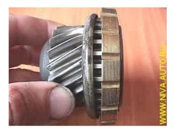
The **synchronizer baulk rings** are cleaned out and examined for deterioration of the tooth tips from both sides:
