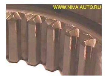
The fork groove facet should be precise, without any burrs.
