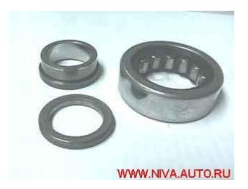
Stretch the plastic needle bearing cage to check its integrity and examine the rollers for pitting or scoring:
