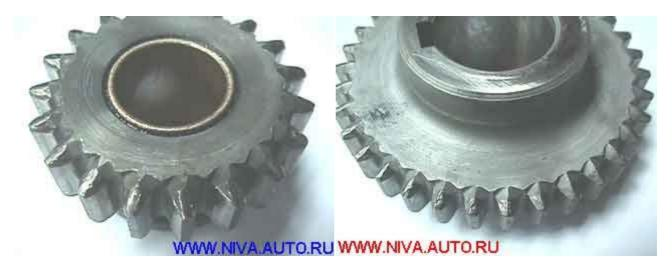
The  $5^{th}$ /reverse gear cluster is checked on presence of all teeth (sometimes the slanting teeth break up) and absence of cracks on them. Also check the small sprocket for damage on the end faces. The bearing inner race should not be removed by the hand's force:
