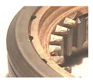
Also the working surface of the sleeve should not have any scores made by the baulk rings:
