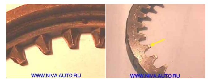
There should not be wear or rub marks on the top part. The left picture shows marks made by contact against the lockring. The marks also tell how strong the baulk ring interacts with the sleeve, in this case the baulk ring sinks deeply and its top face bears against the sleeve teeth (right picture):
