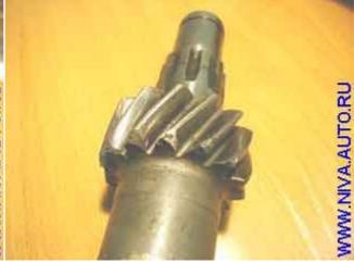
Check the condition of the front and rear end threads. Note (on the left picture) that the 4-speed gearbox countershaft rear end isn't threaded:
