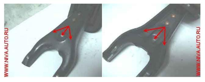
A cracked or worn out fork is replaced by a new one.
