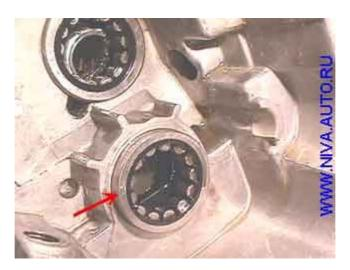
A lot of fragments and debris accumulates in the **gearbox case** front and rear and between the casting reinforcement ribs. Wash all the case thoroughly:
