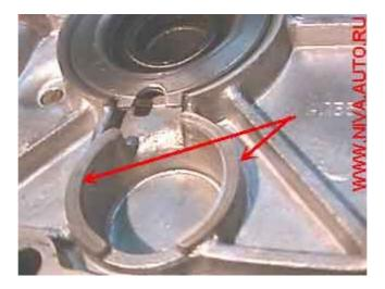
If these tabs are damaged the complete bellhousing must be replaced.
