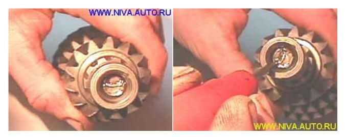
Check the **input shaft** bearing, the  $4^{th}$  gear sprocket, the synchronizer baulk ring and its spring. If there are any remarks about its condition replace the input shaft by a new one.
