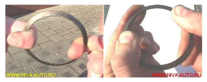
A warped, damaged or broken washer is replaced by a new one:
