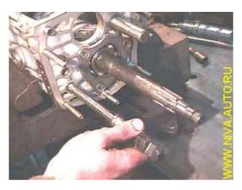
Also check the condition of the detent mechanism surfaces and the shift gates (where the shifting mechanism works). Faulty rails are replaced by new ones.
